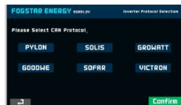
Changing the inverter protocol via the screen.
